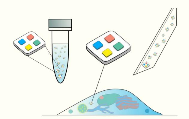
SPAchip®: An intracellular silicon device on which multiple highly concentrated fluorescent probes can be printed to provide intracellular readouts over long culture periods
