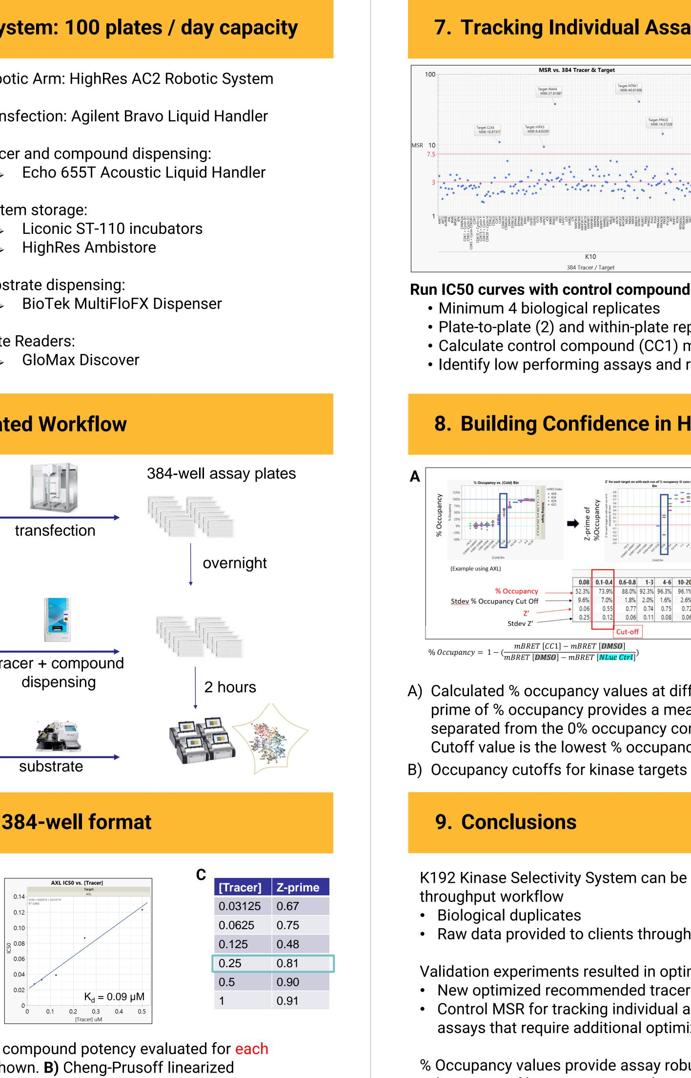
relationship of test compound (CC1) IC<sub>50</sub> versus tracer concentration: IC<sub>50</sub> =  $K_i/K_d x$ [Tracer] + K<sub>i</sub>. C) Z-prime to confirm assay quality at chosen concentration. Choosing tracer concentrations at or below K<sub>d</sub> result in more accurate compound affinity estimates but with lower Z' value and assay window.
